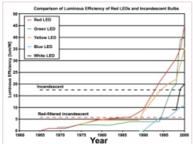
Figure 2. Rise in LED luminous efficiency – adapted from Scientific American, 2001.
