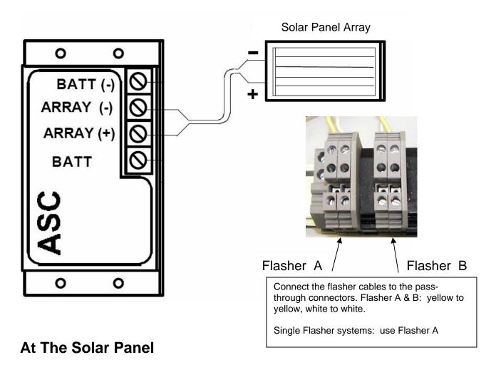
Using a voltmeter check for voltage (17v - 23v) at the terminals, with no wires connected, in the junction box on the back of the solar panel.
