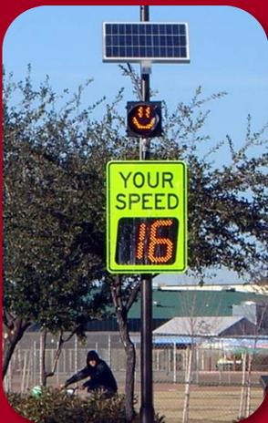
Drivers approaching the SpeedCheck displays at or below the speed limit are greeted with “smiley face” beacon.
