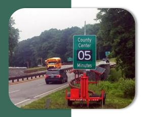
TravelTime<sup>™</sup> is a cost-effective solution for delivering real-time travel information. TravelTime displays the drive time to points ahead, allowing drivers to choose alternate routes.
