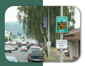
TrafficFlow Manager is a tool for improving the flow of traffic on roadways controlled by successive traffic signals. Drivers tend to accelerate forward when the lights turn green, only to brake at the next light. The ensuing congestion, frustration, and rearend collisions can easily be avoided by giving drivers good information.
