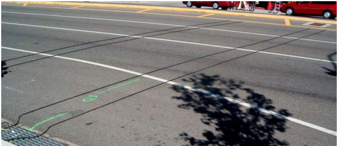
Figure 4-19: Tube Configuration Shown at the Salt Lake City Site
