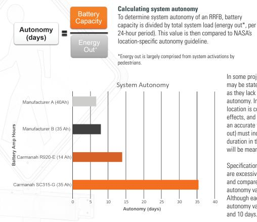
A requirement for a given system autonomy value, without consideration of all the factors that influence autonomy, is not a reliable way to specify any solarpowered flashing beacon system. To ensure a flashing beacon balances both performance and cost, one of the most important factors to identify is location, since the amount of shading affects the amount of power the sun can generate. Read more about shading in **Energy Balance article 4.**
