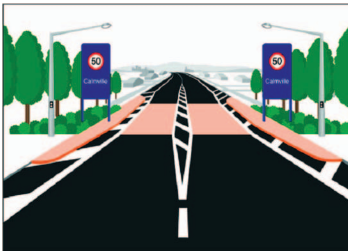
Figure 2-10. Completed threshold (LTSA, 2002).
