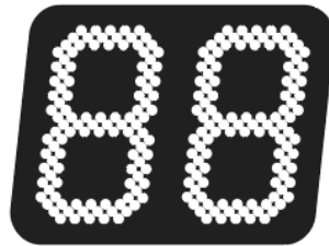
Compliant width-to-height ratio of 0.7
