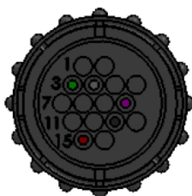
CONNECTOR VIEW FROM WIRE ENTRY SIDE
