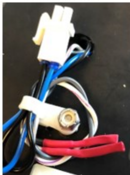
Optional: If present, disconnect strobe connectors.
