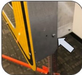
Take note of sign retention bolts, one on each side
