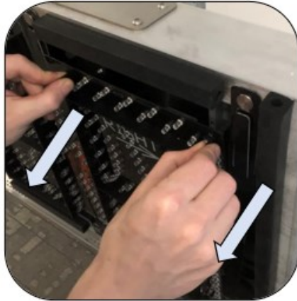
Being very careful not to touch the LED lamps, grasp the circuit board stiffeners at the top.
