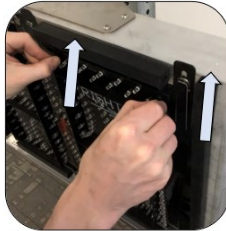
Pull the circuit board toward you about 1/4". When the retainer tabs clear the hanger pins, slide the circuit board upwards.
