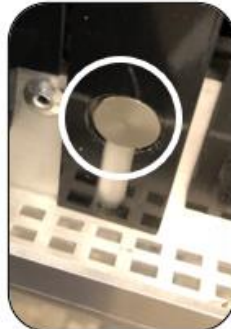
When the top part of the circuit board releases from the upper hanger pins, lower the board to where the cut-outs slip off the lower hanger pins.
