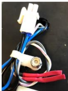
Optional: If present, disconnect strobe connectors.
