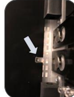
Take note of window alignment stud for re-installation
