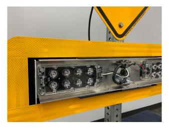
9. Install the light bar front cover and secure using the four Phillips head screws provided with the light bar hardware kit.
