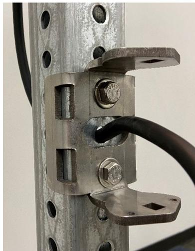
3. Feed the light bar cable through the rubber grommet on the light bar chassis and secure the chassis to the light bar mounting bracket with the fasteners supplied with the light bar. See appendix for additional hardware details.
