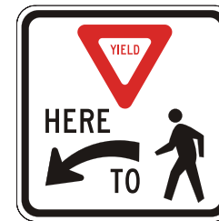
R1-5 yield here to pedestrians sign
