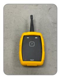
If you are receiving a negative acknowledgement on the transmitter (blinking red LED), try with better line of site or closer distance to the receiver. It is recommended to get a visual of the remote beacon systems to ensure they have been triggered instead of relying on the transmitter acknowledgement LED.
