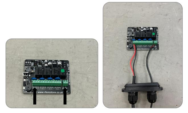
7. Connect the power cable to the barrel connector splitter temporarily. Connect the R838 AC/DC power supply to the splitter. Plug in the power supply to an available outlet to power up the receiver. You should see a red PWR LED on the circuit board showing the board has initialized.
