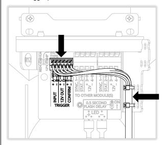
6 Ensure cable ties installed
