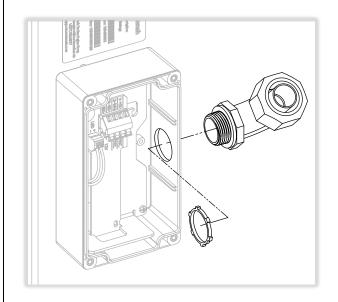
(4)a. Single chevron sign: install conduit fitting onto power module and route conduit. See power module install guide for details.
