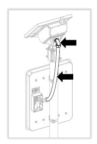
(4) b. Dual chevron signs with adjustable mount kit: install conduit fittings and conduit, see power module and dual mount kit install guides for details.
