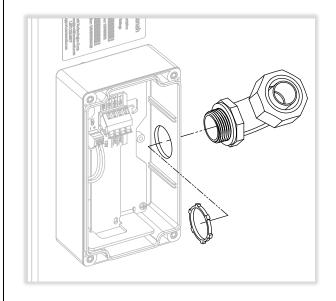
④a. Single chevron sign: install conduit fitting onto power module and route conduit. See power module install guide for details.
