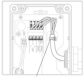
Secure cable jacket with cable tie as shown
