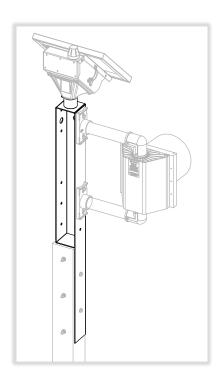
1. Secure wood post mount to corner of wood post with suitable hardware (not included). 5/16" dia. galvanized through-bolts, flat washers, lock washers and nuts are recommended.
