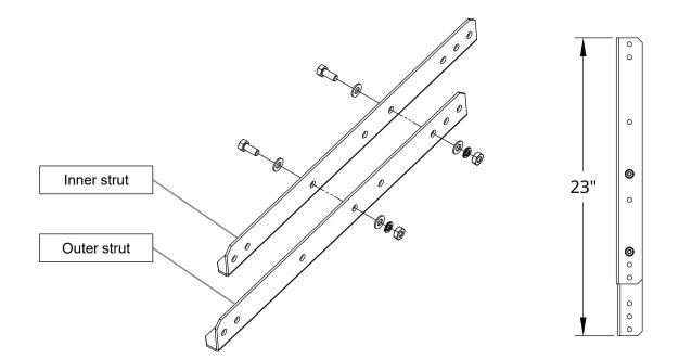
2. Mount one each left and right pivot brackets to lower pole bracket in orientation shown using provided 5/16" hardware. Leave bolts loose.
