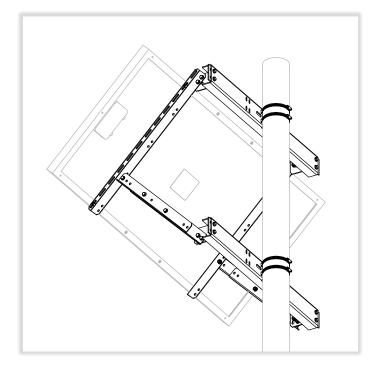
1. Assemble two sets of telescoping lower struts so overall length is 23" using supplied 5/16" bolts, flat washers, lock washers and nuts.
