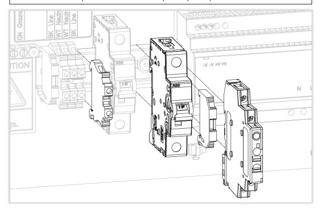
5. Four added components shown in left image below. Slide breaker over against second breaker.
