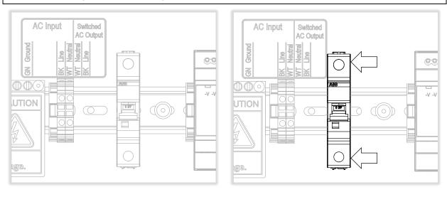
Obtain loose gray terminal block and red jumper from kit. Assemble terminal block into Switched
