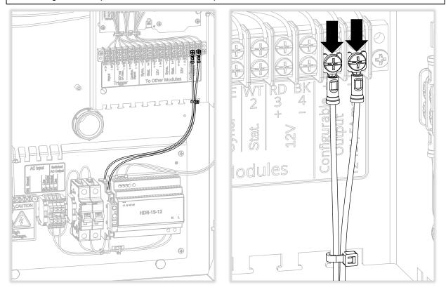
9. Complete relay kit wiring by installing AC input and switched AC output wires.
