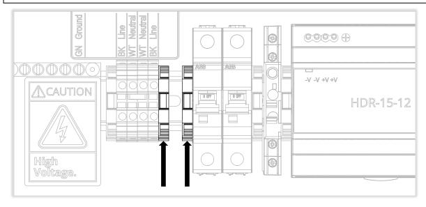
7. Loosen top terminal screw on left breaker. Insert jumper wire from right breaker into left breaker terminal as shown. Tighten terminal screw ensuring both wires are secure. Install provided cable tie as shown around relay and power supply wires.
