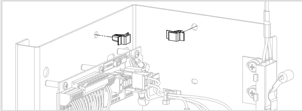
3. Route and secure door switch wires with cable ties provided. Leave cable ties loose and untrimmed.
