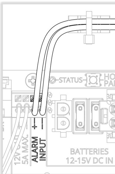
4. Remove insulation from pre-stripped switch wires and insert into power module Alarm Input terminals, using a suitable tool to depress terminal buttons. Tighten and trim cable ties.
