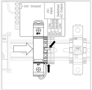
3. Install SPD with longer white wire next to first SPD. Install terminal block next to existing Neutral terminal block. Push both SPD and terminal block snuggly against other components. Ensure red jumper is installed between two terminal blocks.
