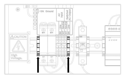
5. Connect ground wires from top of SPDs to neutral bar as shown, tighten terminal screw and pull test wires to ensure they are secure.
