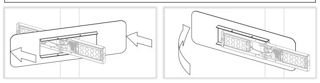
3. Center backplate with light bar chassis and slide light bar cover back on.
