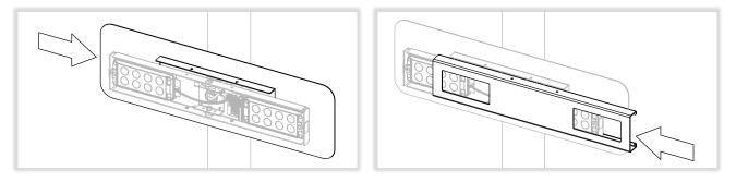
4. Pull backplate forward over light bar cover. Align holes in backplate, light bar cover and captive nuts on chassis underneath. Install all four screws loosely before tightening.
