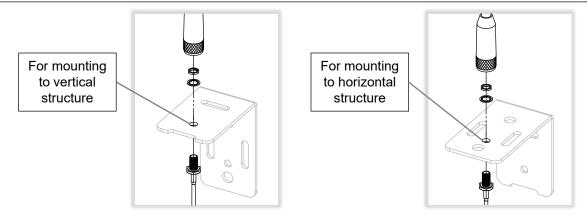
3. Remove antenna, washer and O-ring from power module and connect remote antenna cable in its place. Wipe off any excess grease that may have been pushed out of connector and apply provided sealant tape over connection.
