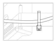
4. Secure any slack in the cable as required to limit strain on connections.
