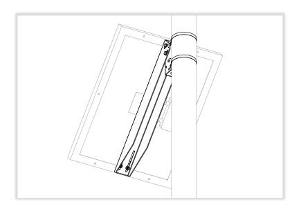
1. Fasten support arm to solar panel frame following mount manufacturer's instructions. Ensure solar panel is centered on mount bracket.
