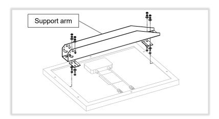
2. Install mounting bracket on pole following mount manufacturer's instructions. Ensure bracket faces south (in North America).
