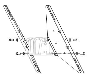
2. Fasten sheet metal brackets to casting with four bolts and flat washers.
