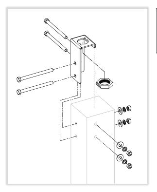
Secure bracket to corner of wood post with suitable hardware. 1/2" dia. galvanized through-bolts, flat washers, lock washers and nuts are recommended. Insert hex nut under bracket aligning nut thread with hole in bracket.
