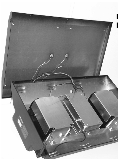
Figure 16: Solar Engine top cover showing notch for antenna assembly
