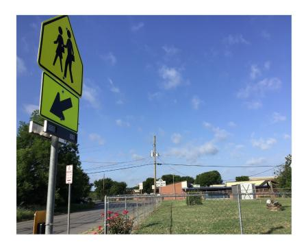
Even the marked crosswalk at the intersection of Hines and Lucas is unsafe. There are only two stop signs, and these are on Lucas and not Hines, where the crosswalk is located. The crosswalk paint is faded, signage is easily obscured by trees and parked cars, and there is just one curb ramp, which itself is too narrow to accommodate people with disabilities.
